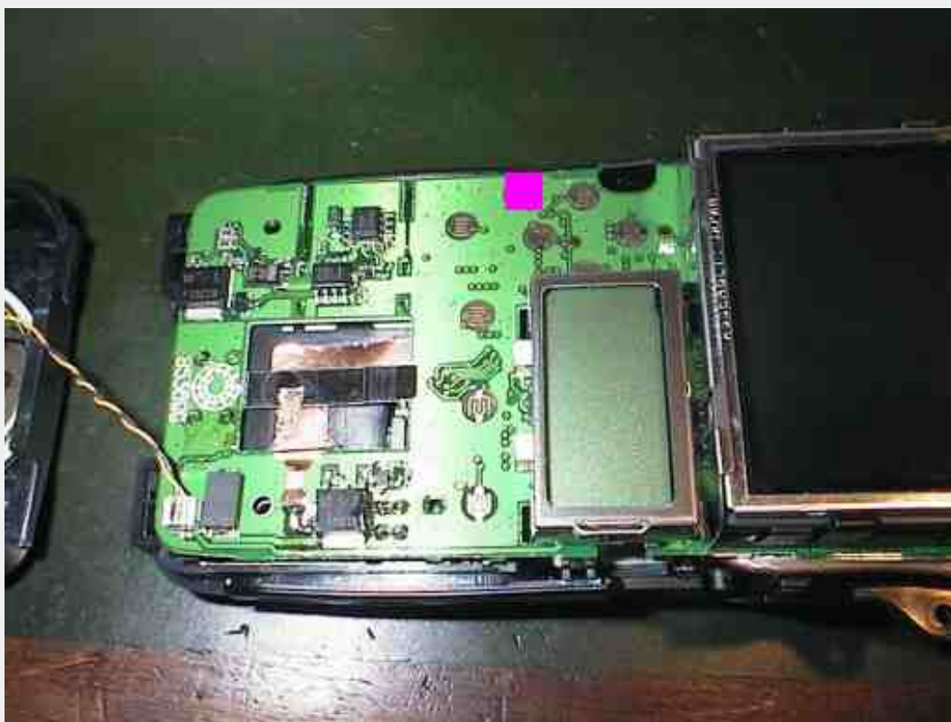
Fig. 2 Remove the speaker leads and the screw marked
