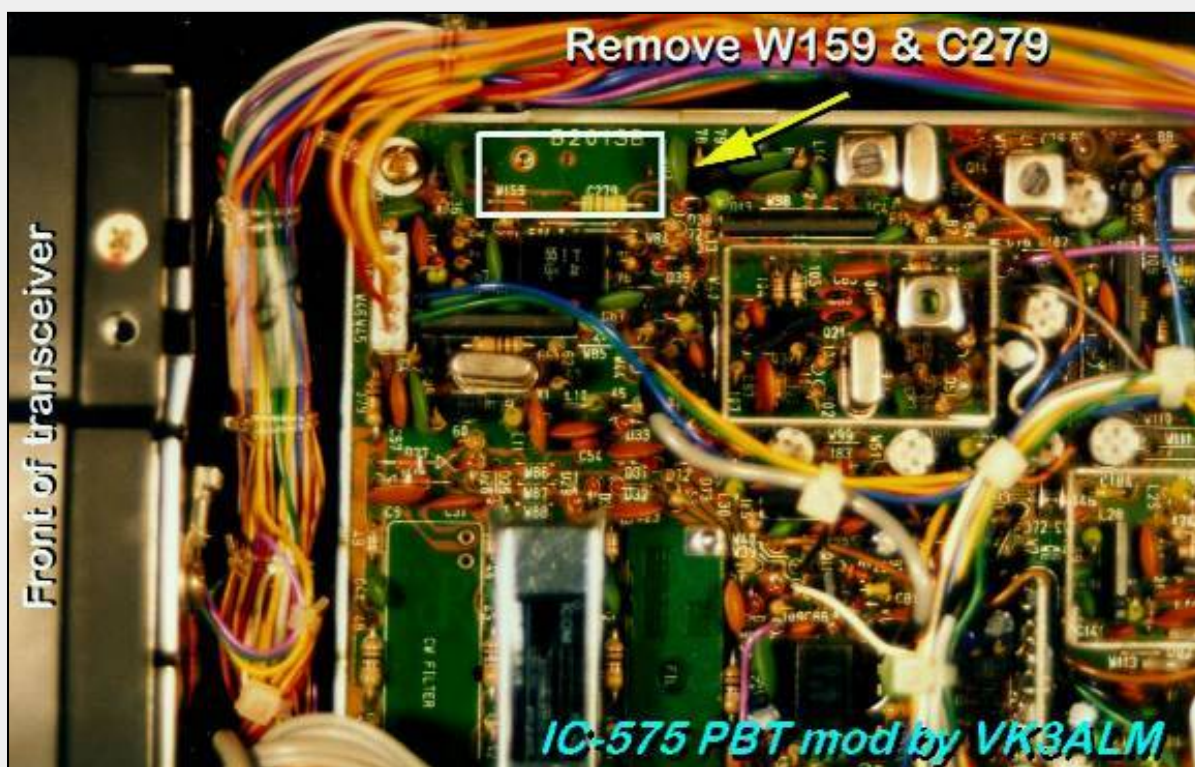
Picture 2 - Location of filter area on Main Unit PBA
