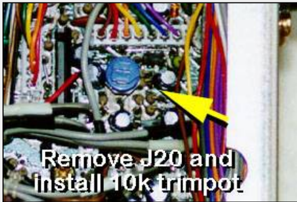
Picture 3 - 10k trimpot fitted to where J20 used to be.
